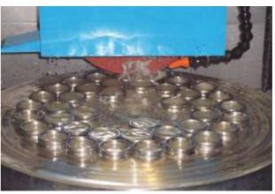
The face- and step-processing of flat rotationally symmetric work pieces is in many cases easier than with a classical cylindrical grinding machine. Especially heavy work pieces can easily be loaded and positioned onto the working table. Serial parts can be worked much economically as with a classical surface grinding machine, as the acceleration at the reverse points is not existent.
