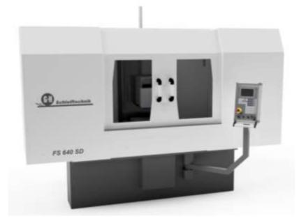
This machine was conceived especially for individual and small-lot production. In a workshop, it is necessary that surface grinding machines are easy to use. Process modifications must be easily realisable. The SD-control was developed for this scope of operations. Especially for adjustment work, the infeed can be made with µm-precision by means of the electric manual wheel – analogue to the manual wheel of a hand-controlled machine.
