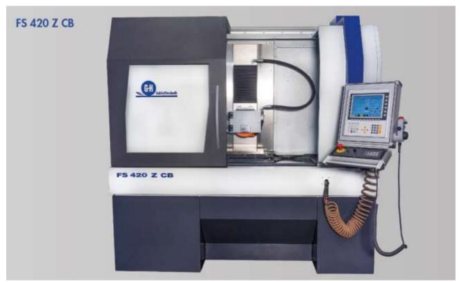
This machine was conceived especially for individual and small-lot production. In a workshop, it is necessary that surface grinding machines are easy to use. Process modifications must be easily realisable. The CB-control was developed for this scope of operations. Especially for adjustment work, the infeed can be made with  $\mu$ m-precision by means of the electric manual wheel – analogue to the manual wheel of a hand-controlled machine.
