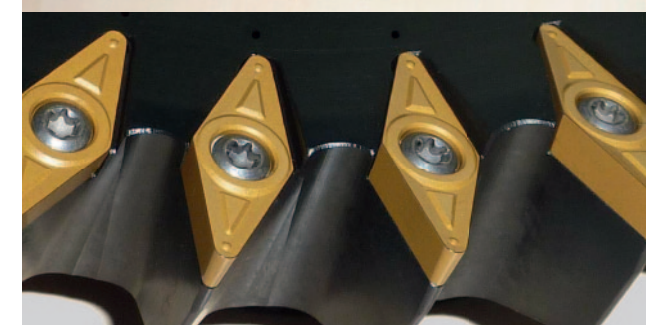
Power-Skiving cutter with carbide inserts.
